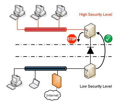
Data integrity is maintained by using a custom-developed, proprietary communications protocol that has intelligent error correcting codes. Logging all transfer activities on both sides of the transaction ensures that all 'events' during a transfer are tracked and timed, and abnormal activities are detected and reported.
